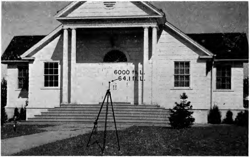
Fig. 8. Illustration of the use of the adaptometer for field work.
